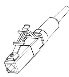
The MIL LC Connector have housing and clip in metal, which increase endurance in sub-zero temperatures compared to plastic designs that will become fragile. The metal housing also offers improved positions accuracy over time. When connected and disconnected multiple times, the plastic housing will tear out easier, compared to MIL LC Connector with metal housing and clip.
